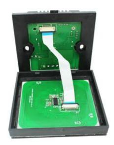
(2) remove the cable. Pull the locking of the terminal transposon, and then you can slowly remove the cable, as shown below:
